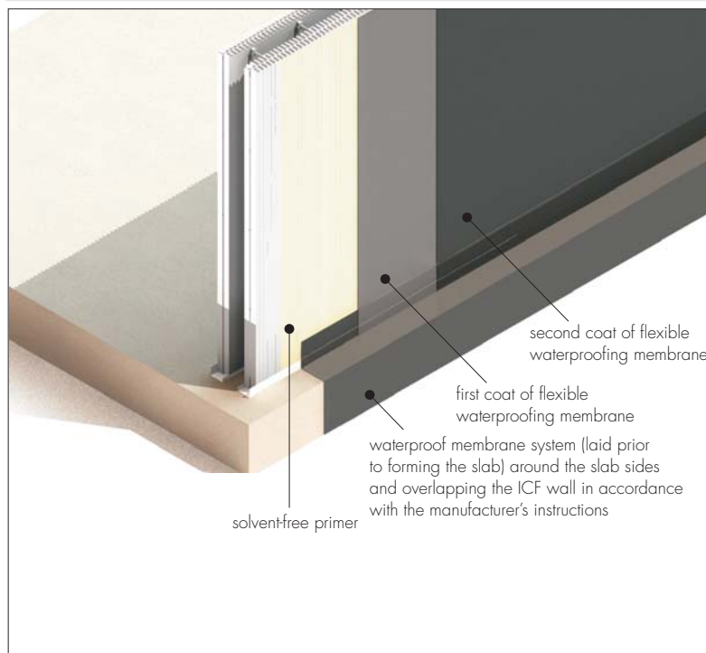
Figure 3 Typical basement detail with external waterproofing membrane
